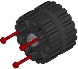
Step 7: Perform these steps with four Round Double Boss Nubs (am-3413a) and two double boss Dbore nubs (am-3215a), to create six total pulley assemblies.
