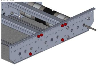
**Step 21**: Place the second Outside Plate Assembly flat resting on the screw heads.
