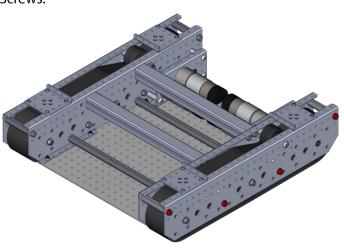
**Step 27**: Work your way around the chassis, ensuring all other 1/4-20 Thread Forming Screws have been fully tightened.
