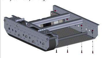
**Step 20**: Finish tightening the 1/4-20 Thread Forming Screws.
