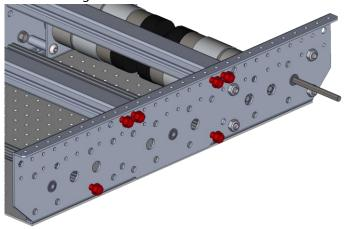
**Step 19**: Secure the Belly Pan to the second Inside Plate Flanges, using two 6-32 x 0.5 in. Screws and two 6-32 Nylock Nuts per flange.
