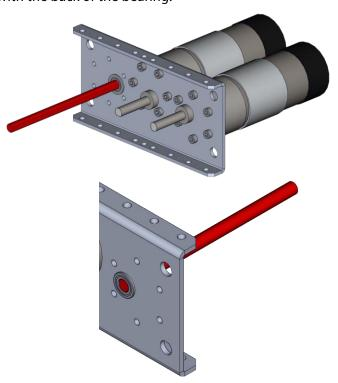
**Step 5**: Place a 0.50 in. OD x 0.242 in. ID x 0.354 in. Long Aluminum Spacer (am-3426) onto the 6 mm D shaft, flush against the bearing.
