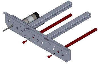
**Step 12**: Holding the Inside Plate Assembly by the left peanut, guide the Inside Plate and Outside Plate Assemblies together. Start by lining up the PicoBox output shaft with the D Bore Pulley Assembly. Line up the remaining three axles. Open ended wrenches can be used to persuade shafts and pulley assemblies to their correct position.
