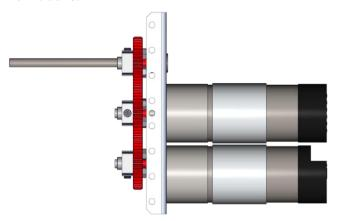
**Step 9**: Tighten the set screw for each Gear-Nub Assembly with the 3/32 in. Allen Driver.
