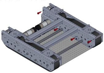
**Step 25**: Use four 6-32 x 0.50 in. Socket Head Cap screws and four 6-32 Nylock Nuts to secure the
