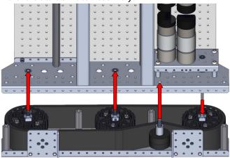
**Step 23**: Loosely secure the assemblies with two M6 Nylock Nuts and one M8 Nylock Nut onto their respetive axles.
