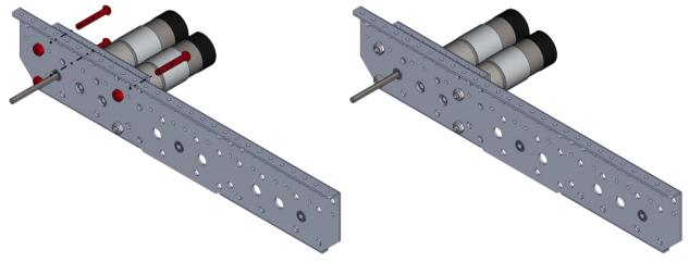
**Step 4**: Use the same steps, mirrored, to create and combine the opposite handed PicoBox Gearbox and PicoBox-Inside Plate assembly.
