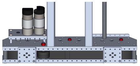
**Step 14**: Secure the 4x4 Chassis Plates to the Inside Plate with two 6-32 screws and two 6-32 Nylock Nuts each.
