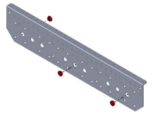
**Step 4**: Install three bearings into an Inside Plate (am-3392\_Inside.) All bearings are installed with flanges opposite the long continuous plate flange.
