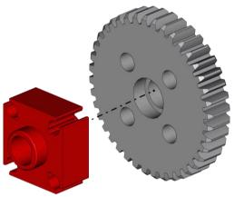
**Step 3**: Ensure the 10-32 set screw is pre started into the nub with
