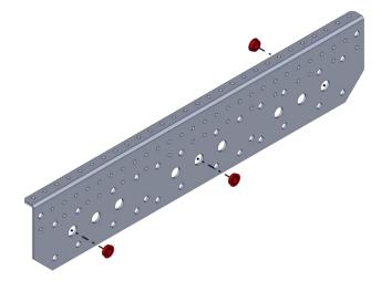
**Step 5**: Mirror the bearing installation on the remaining inside plate with three additional 6 mm bearings.
