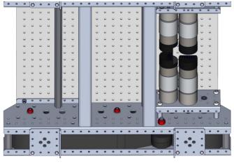
**Step 24**: Loosely tighten the Outside and Inside Plates together with four 1/4-20 Thread Forming Screws into the four 63 mm Churros.
