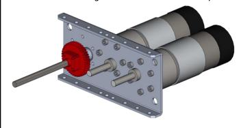
**Step 7**: Add two more Gear-Nub Assemblies to the gearbox, one on each NeveRest Gearmotor Shaft.
