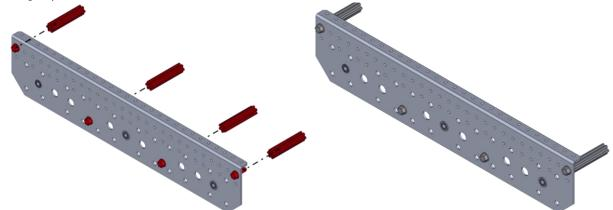
**Step 2**: Secure two 4x4 Chassis Plates (am-3393) to the Outside Plate using 6-32 x 0.50 in. Thread Patch Hex Head Screws (am-1563) and 6-32 Nylock Nuts (am-1419.) Use two nuts and screws per plate. These can be placed or moved to any location you prefer, keeping in mind clearance is needed for the tensioner pulley. A 5/16 in. wrench will hold the Nylock Nuts.
