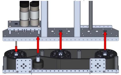
After joining, the end of the PicoBox output shaft will be flush with the left bearing on the outside plate.
