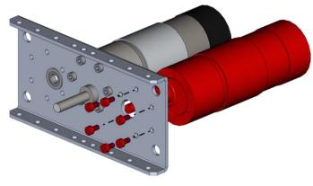
**Step 4**: Insert the 100mm Long 6mm D Shaft (am-3226-100) into the flanged bearing. The shaft must be flush with the back of the bearing.
