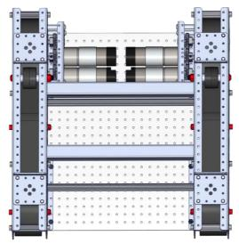
**Step 29**: Double check that all Nub Set Screws have been tightened.
