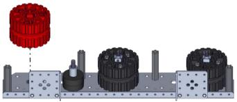
**Step 8**: Place the TreadRunner Tread (am-3963) around the three main pulley assemblies, and under the tensioner pulley.
