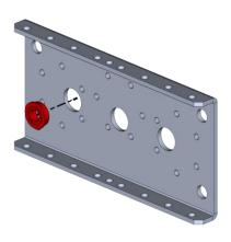
**Step 2**: Secure the first NeveRest to the plate using six M3-0.5 x 5mm Socket Head Cap Screws (am-1443.)
