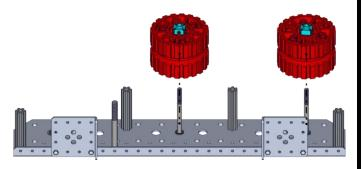
**Step 6**: On the tensioner axle, place a 0.75 in. Long Aluminum Spacer (am-1541) followed by an 8 mm Bore Roller (am-3979), and a second 0.75 in. long spacer.
