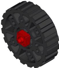
**Step 3**: Ensure the 10-32 set screw is pre started into the nub. (Lost set screws? Get more as am-1342.)
