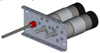
**Step 6**: Place one of the Gear-Nub Assemblies onto the 100 mm D Shaft. The gear will be flush with the spacer.
