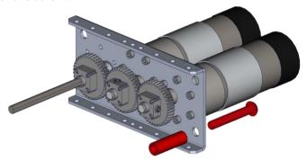
**Step 2**: Join the Inside Plate and PicoBox Assembly. Insert the 1/4-20 Button Head Cap Screw into the fourth hole from the left on the bottom row of holes of the Inside Plate. The PicoBox Output Shaft will insert through the left bearing of the plate. Finger tighten a 1/4-20 Nylock Jam Nut (am-1102) on the 1/4-20 Button Head Cap Screw.
