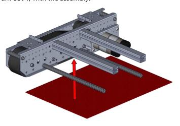
**Step 17**: The Belly Pan is secured to each flange with two 6-32 Socket Head Cap Screws and two 6-32 Nylock Nuts. The hardware location is based on preference
