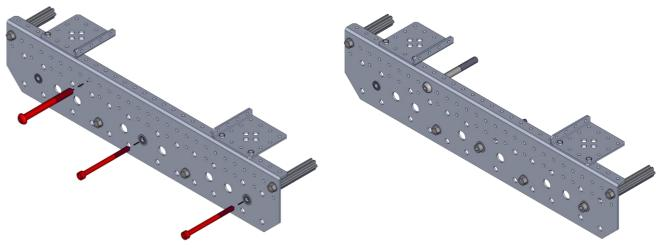
**Step 4**: Lay the assembly flat on the screw heads with the top flange towards you.
