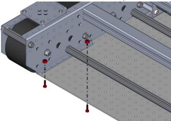
**Step 18**: Using six 1/4-20 Thread Forming Screws, loosely attach the second Inside Plate Assembly to the 11.25 in. Long Peanut and Churro.
