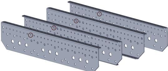
**Step 2**: Install three 6 mm x 12 mm Flanged Bearings (am-3377) into an outside plate (am-3392\_Outside). The left most bearings' flange is on the same side as the plate flange. The middle and right bearing are installed from the opposite side.
